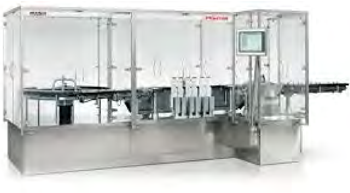
Barrier Fill Line Process
