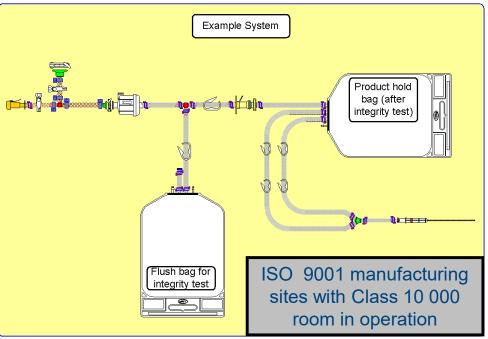
Biocontainers and critical components tested at 100 %
