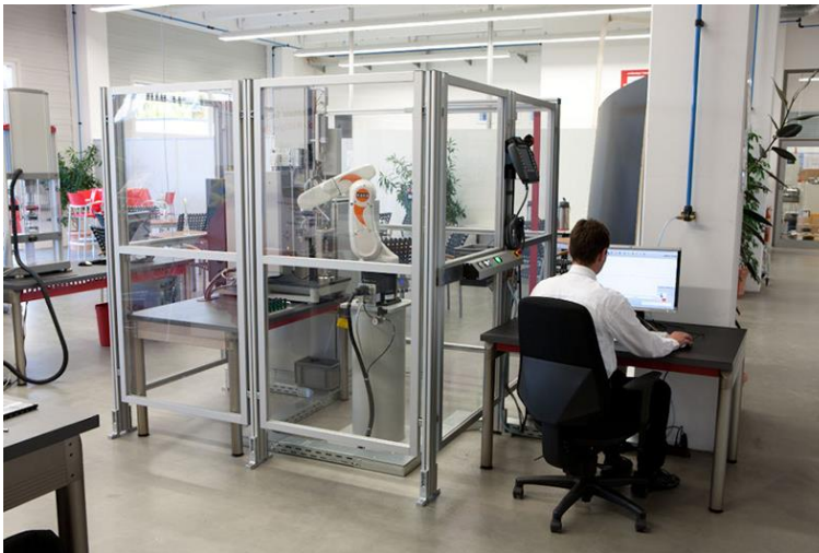
Robotic Testing System ,roboTest R' with torsion-testing machine 2.5 kN for functional-test on insulin-pen
