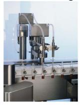
Cartridge for pen system Hole for filling  $\emptyset$  (inner) = 3,15 ± 0,2mm
