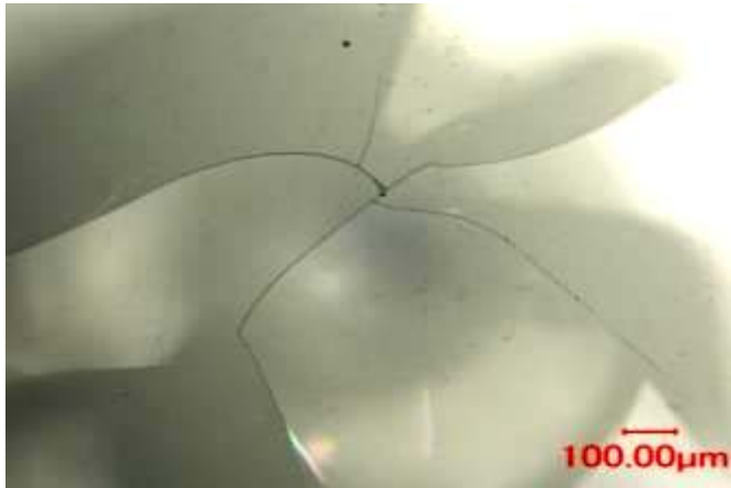
Laser Exit (interior surface )
