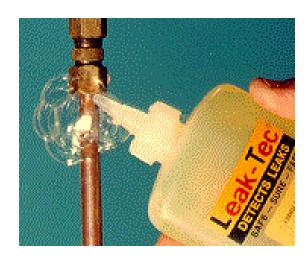
Surfactant solution used at suspected leak site
