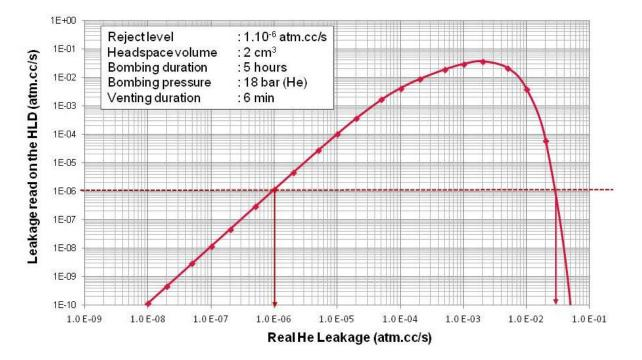
$\rightarrow$  In particular cases, the measured Helium leakage could be the same for a large leak or a fine line.
