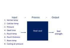
This type of experiment involves changing one or more inputs and measuring the resulting effect on one or more outputs
