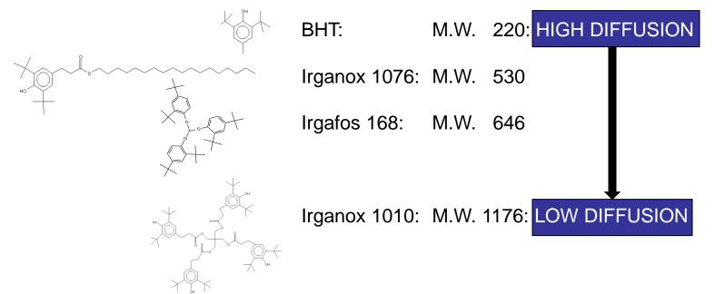
Polymer Additive DEGRADATION INTO SMALLER MOLECULES  $\rightarrow$  FASTER DIFFUSION OF DEGRADANTS
