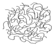
Interstitial space (between polymer chains) Total Volume of the Polymer
