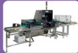
Semi-Automated Visual Inspection (SAVI)
