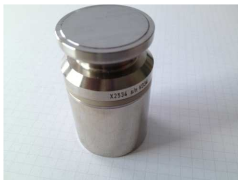
Freeze Dryer Logger - -85C to +140C
