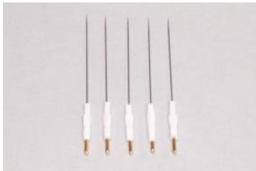
Tungsten needles for particle picking
