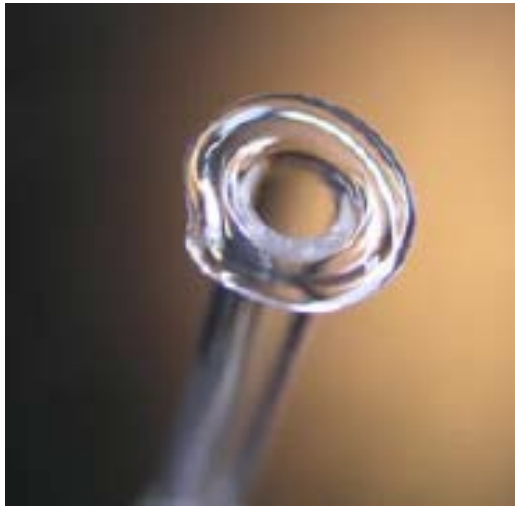
Fingertip not properly tooled
