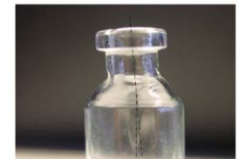
The finish and plane of the seal surface is not perpendicular to axis of the body.
