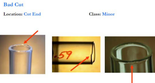
Poor cut resulting in an irregular glazed end
