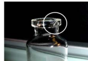
Small particles or fragments of glass adhered to the interior or exterior surface of the vial.
