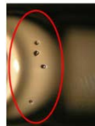
Small particles or fragments of glass adhered to the interior or exterior surface of the vial.
