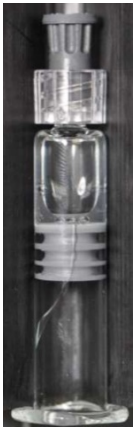
Cracks going through the glass wall
