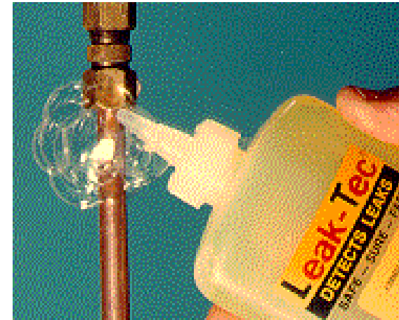
Surfactant solution used at suspected leak site
