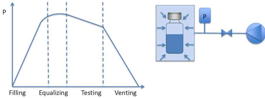
Pressure decay => pressure levels between 300 – 900 mbar
