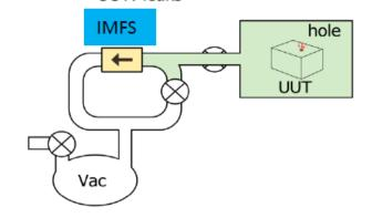
4 Test - Steady flow thru leak
