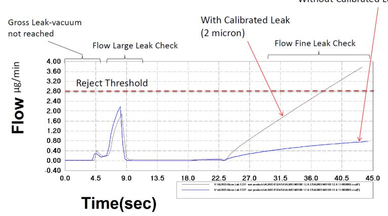
Note: The Smaller Defect Size Mass Extraction is set to detect (Limit Of Detection)- the lower is the customer risk.
