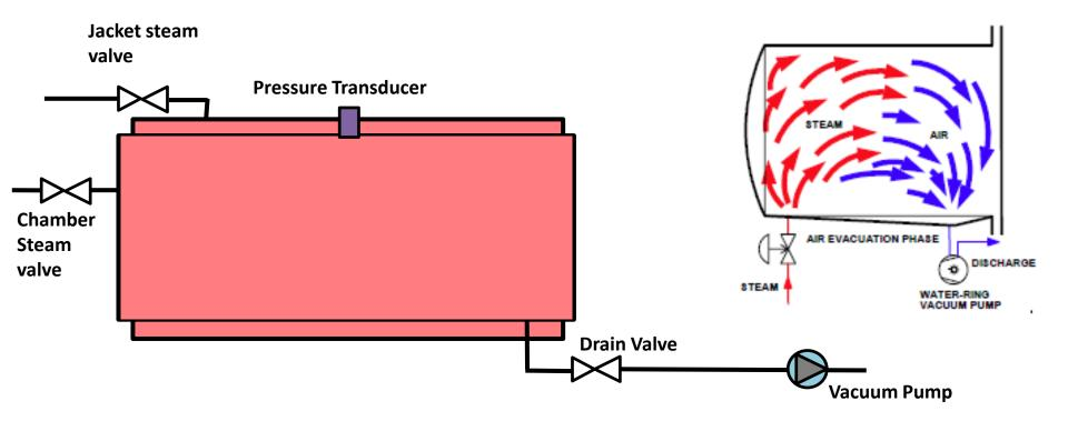
Steam is injected into the chamber displacing the air, the vacuum pump extracts both steam/condensate and air from the chamber.
