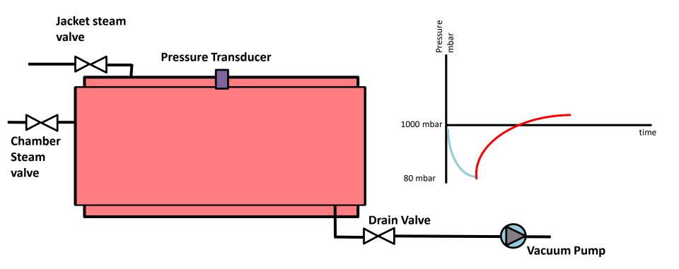
Steam is injected into the chamber displacing the air, the vacuum pump extracts both steam/condensate and air from the chamber.
