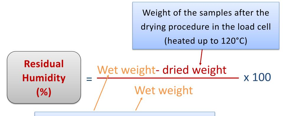
Samples weight before heating procedure (after sterilization treatment)
