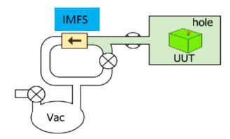
3 Stabilize - Leak: increases P<sub>chamber</sub>- IGLS: begins flow
