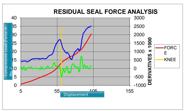
The compression curve (red) is a combination of the viscous and elastic responses to the stress from tester load. "The knee"(yellow) is where additional deformation occurs. An algorithm is applied, using the 1st (blue) and 2nd (green) derivatives to accurately identify that knee.
