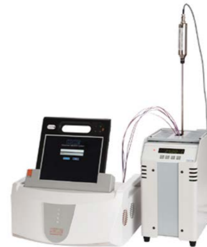
Construction of a recorder system including a temperature standard
