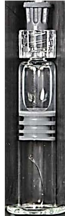
Crack not touching the drug
