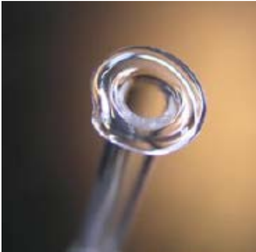
Fingertip not properly tooled
