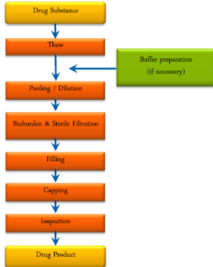
Fig. 3. Flow chart of a standard MAB manufacturing process.
