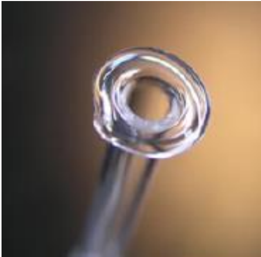
Fingertip not properly tooled
