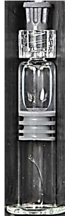
Crack not touching the drug
