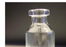
The finish and plane of the seal surface is not perpendicular to axis of the body.
