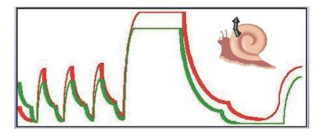
For loads that cannot tolerate rapid pressure changes, such as filters, membranes, stoppers in bags, a modified pulsed air removal process is required.
