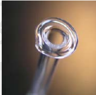
Fingertip not properly tooled
