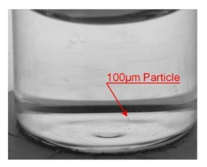
Threshold study of various particle sizes will orientate you in selection of particle size in your true defect zone. Take into consideration:
