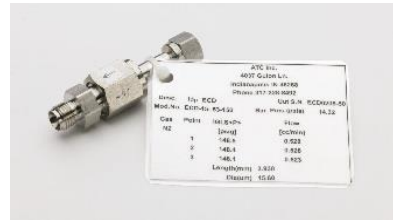
Calibrated leak (inside)
