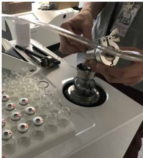
5/. Installation of the rubber plug
