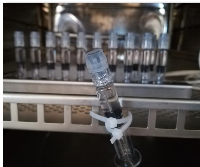
Sample with the TC inserted directly inside the syringe
