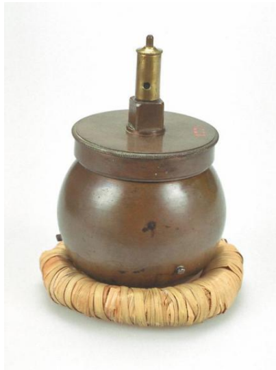
Denis Papin "Digester" Museum for the History of the University of Pavia (Object from the collection of Alessandro Volta)
