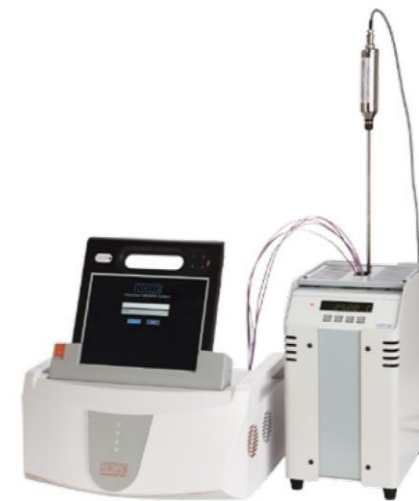
Construction of a recorder system including a temperature standard
