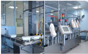
Passive open RABS on a syringe line
