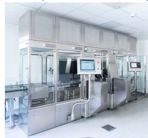
Active open RABS on Freeze Dryer
