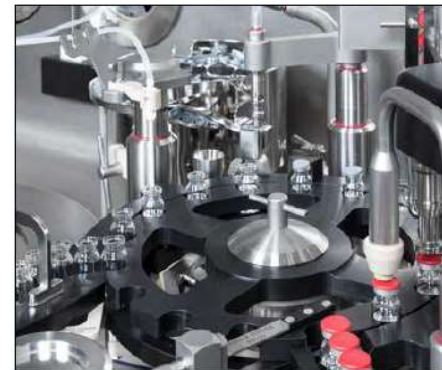
KSF 5105 – Fully automatic vial filling and closing
