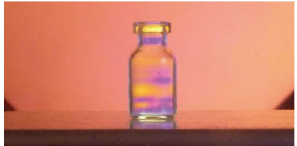
Residual stress in the vial after forming
