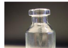
The finish and plane of the seal surface is not perpendicular to axis of the body.
