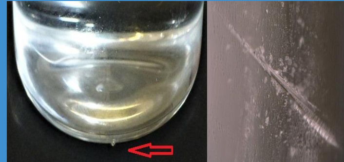
Phenomenon B – „Heel Stickers“/Scratches
