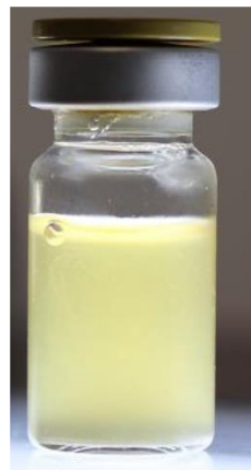
Turbid vial identified during inspection with a passed-through crack that caused a loss of integrity
