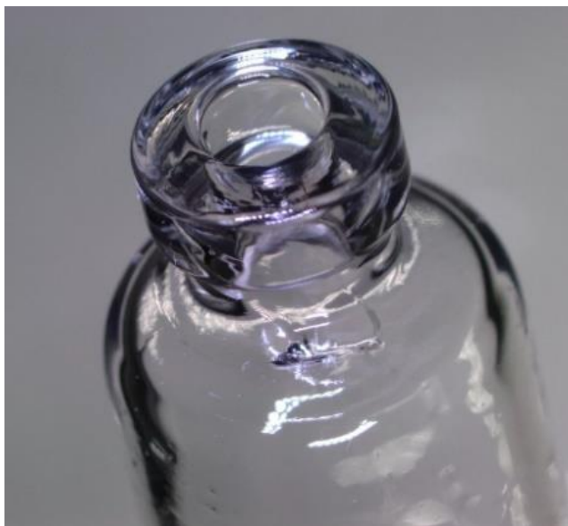
Glass defect with a hole in the shoulder area, causing leakage during use
