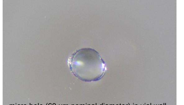
micro hole (60 µm nominal diameter) in vial wall frontal
