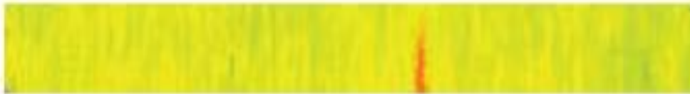
Side seal with 0.75mm defect
