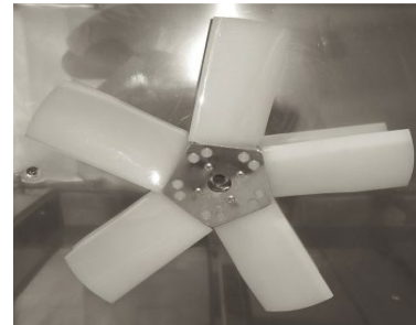
Magnetic coupling propeller
