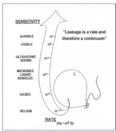
Smallest leaks only allow gas flow
