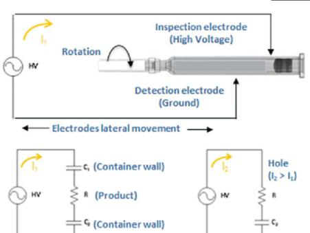
A high voltage is applied on the container to pass through the inspection electrode.
