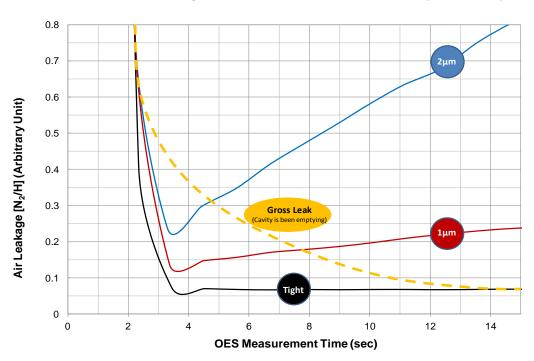
The air leakage corresponds to the intensity ratio [N<sub>2</sub>/H]
