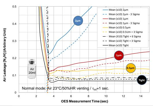
The Air Leakage raw signal corresponds to the intensity ratio  $[N_2/H]$ .
