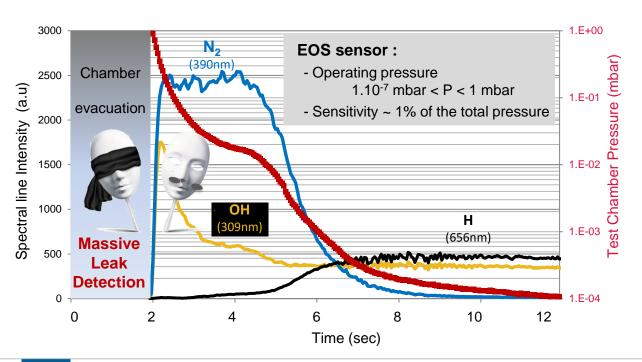
The air  $(N_2)$  inside the test chamber can be easily evacuated using vacuum pumps.
