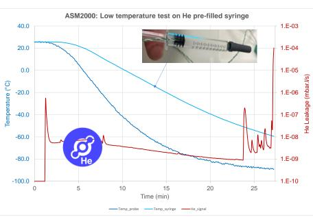
→ Loss of integrity around -60°C can be detected with both test methods O.E.S. and Helium
