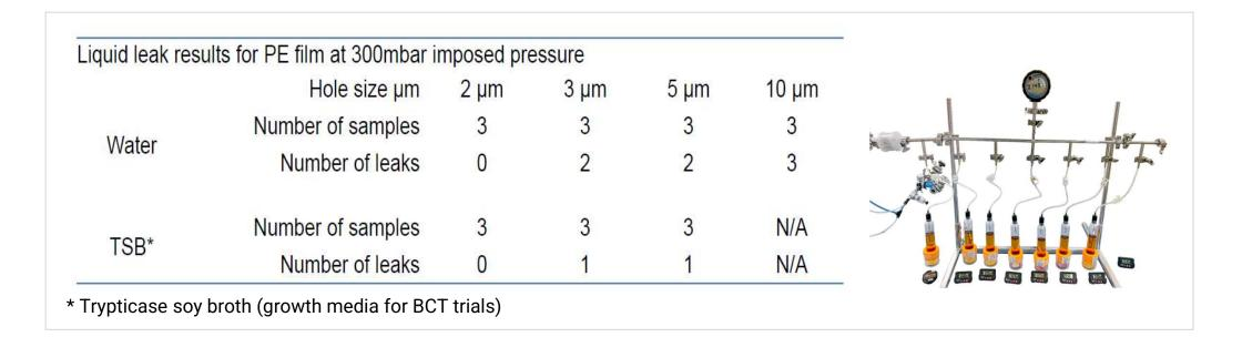
Liquid tests on film show no leaks on 2µm defects at 300 mbar
