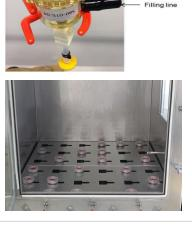
Microbial aerosol tests on 300 film samples show no ingress for 1µm defects at 300 mbar
