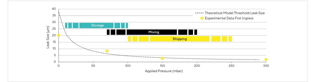
2 micrometers is the MALL for liquid leaks and microbial ingress for all use-case conditions up to 250 mbar
