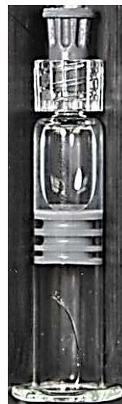
Crack not touching the drug
