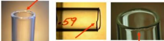
Poor cut resulting in an irregular glazed end
