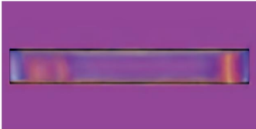
Residual stress in the tube ends of non annealed glass after closing (red = tensile stress, blue = compressive stress)
