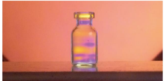
Residual stress in the vial after forming
