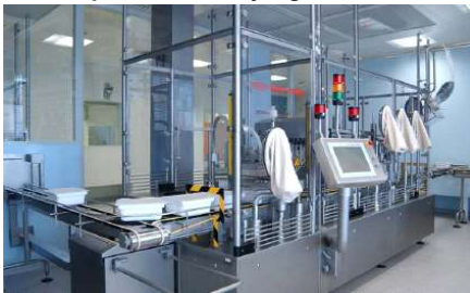
Passive open RABS on a syringe line
