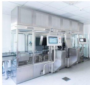
Active open RABS on Freeze Dryer
