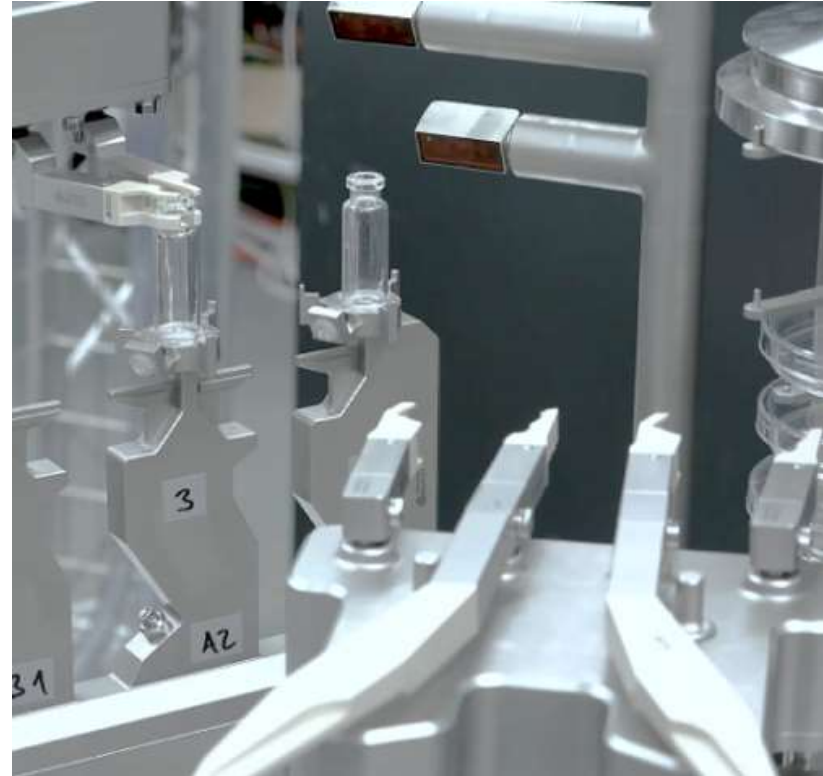
First Air – Refers to filtered air that has not been interrupted prior to contacting exposed product and product contact surfaces with the potential to add contamination to the air prior to reaching the critical zone.
