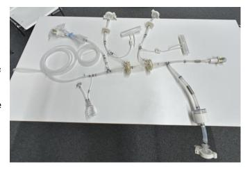
Another proposal discussed in group 1 for difficult to filter products: put two filters in parallel. If one filter starts clogging switch to the second filter.
