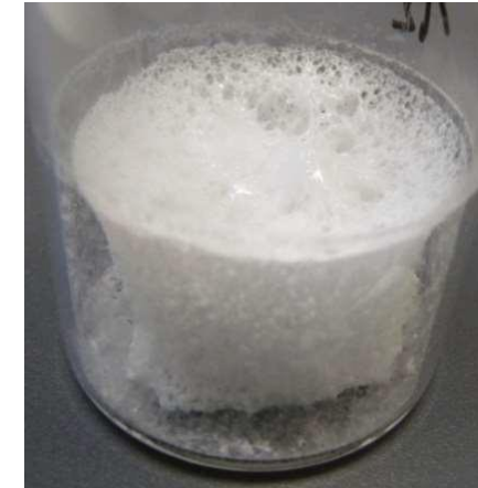
severe collapse / melt-back
