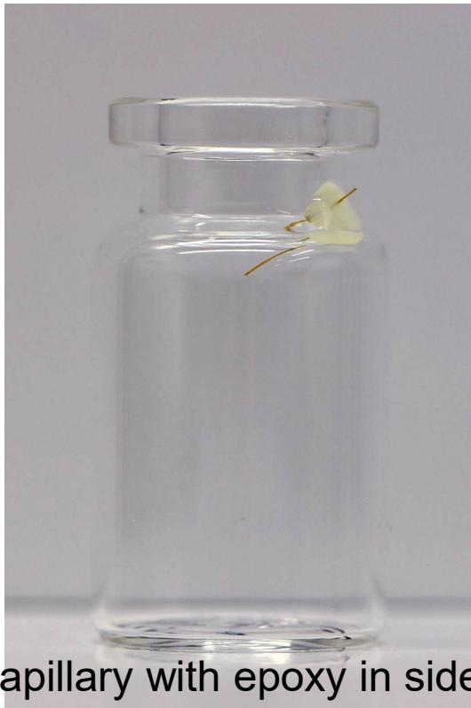
Capillary with epoxy in sidewall
